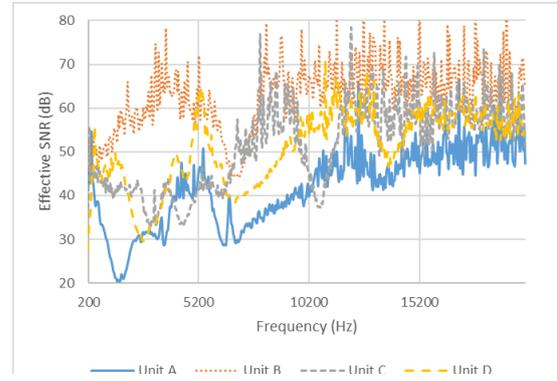
Figure 3. Effective SNR of units under study due to ghost current.
